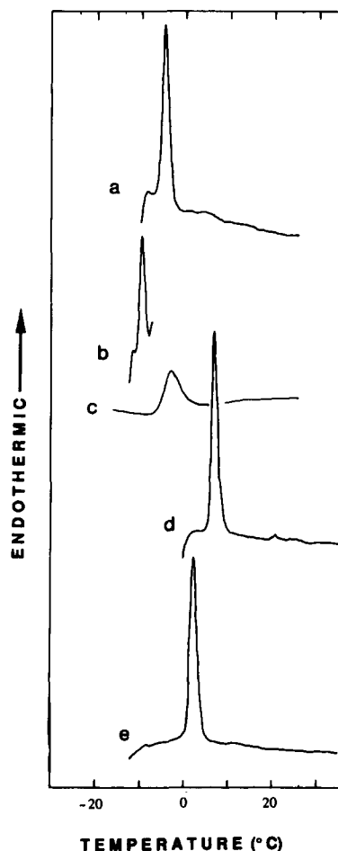
Fig. 1. DSC thermograms at a heating rate of 5 ^\circ\text{C}/\text{min} of (a) POPG; (b) POPG/PMB 5:1 (m/m); (c) POPG in glycerol; (d) SOPC in distilled water; (e) SOPC in glycerol. Different amounts of lipid were present in each case so the peak areas cannot be compared.
